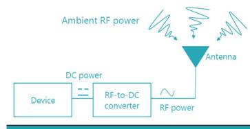
Electromagnetic (EM) waves carry energy, but it is challenging to harvest it in buildings. EM power is relatively weak for energy harvesting, and architectural constraints hamper the propagation of waves. The following challenges will be tackled in this project:
