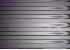
Inkjet Printed Co-Planar Supercapacitor Electrodes for energy storage (to be integrated with RF energy harvester)
