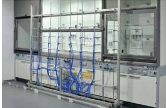
EN 14175-6 type tested fume cupboard control in acc. with 5.4 Measuring in the outer measuring level
