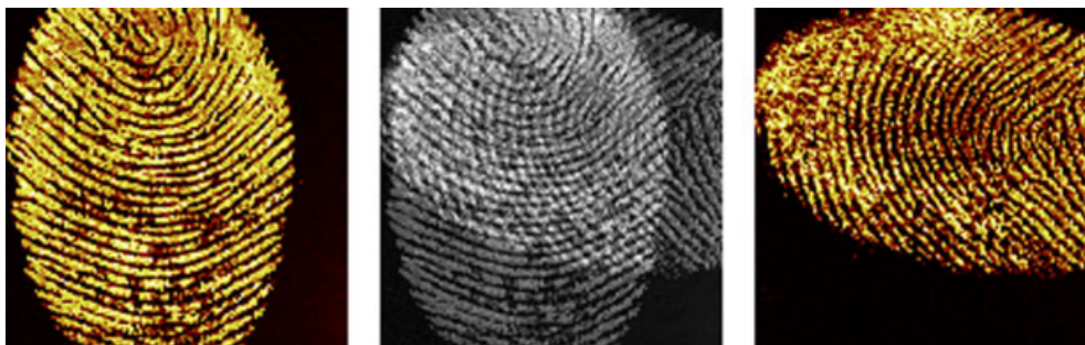
Figure 3. 15 \times 15 \text{ mm}^2 , 128 \times 128 resolution ToF-SIMS negative ion images of two overlaid finger prints on a polyester/polyurethane primer coating.
