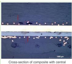
piezo-sensor and conducting wire mesh.
