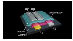
One of the breakthroughs is the MMT's immunity to parasitic effects that reduce a transistor's capacity to produce uniform, repeatable signals. These have hindered traditional "floating gate" designs ever since their invention in 1967, but this new structure promises efficient analogue computation for robotic control, AI and unsupervised machine learning.
