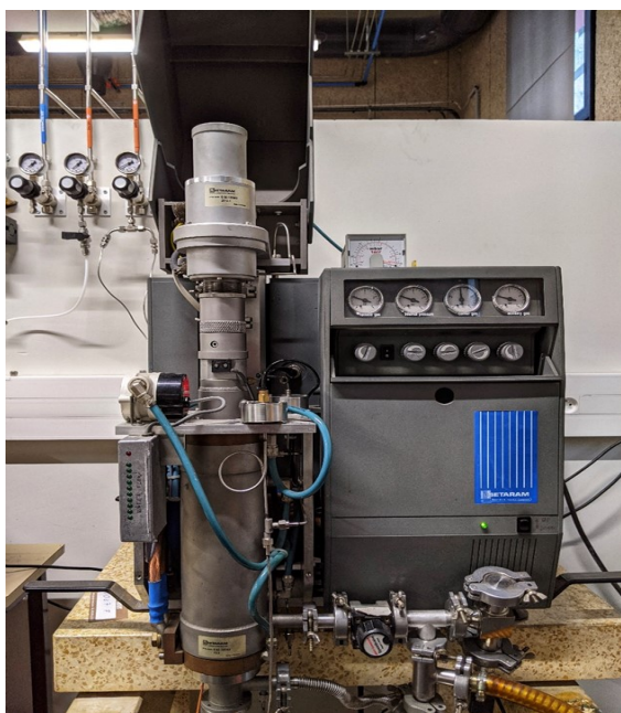
Fig 1: Dilatometer set-up for preliminary sintering experiments
