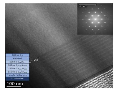
Transmission electron microscopy (TEM, Thermo Scientific Talos F200I) image of a multi-quantum-well (MQW) structure grown via molecular beam epitaxy (MBE). The fast-Fourier transform (FFT, in top-right corner) of the Ge buffer layer evidences the epitaxy growth. The lamella was prepared/polished from a wafer using a xenon plasma focused ion beam (Xe-PFIB, Tescan FERA3).
