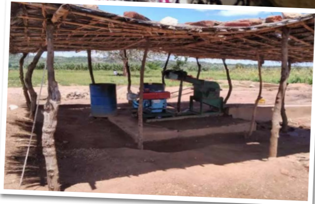
Crushing machine used in ASM
