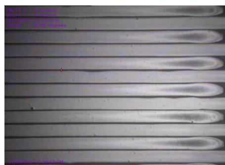
Inkjet Printed Co-Planar Supercapacitor Electrodes for energy storage (to be integrated with RF energy harvester)
