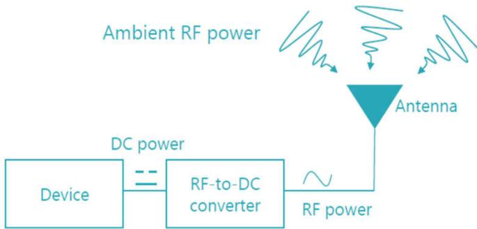
Electromagnetic (EM) waves carry energy, but it is challenging to harvest it in buildings. EM power is relatively weak for energy harvesting, and architectural constraints hamper the propagation of waves. The following challenges will be tackled in this project:
