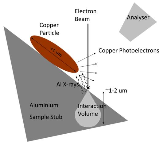
The electron beam strikes the aluminium close to the particle, generating X-rays that in turn, excite photoelectrons from the sample to be analysed.
